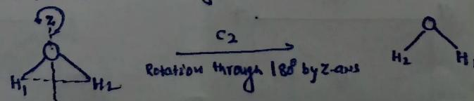
If  $C_2$  is applied in succession i.e. rotation by  $360^\circ$  in  $H_2O$  molecule, we will get identity operation (E) because it will bring back to the original configuration.
